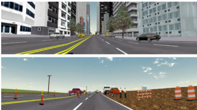
STISIM 3.0 driving simulator city and highway scenarios
